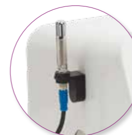
Temperature and Relative Humidity Sensor
