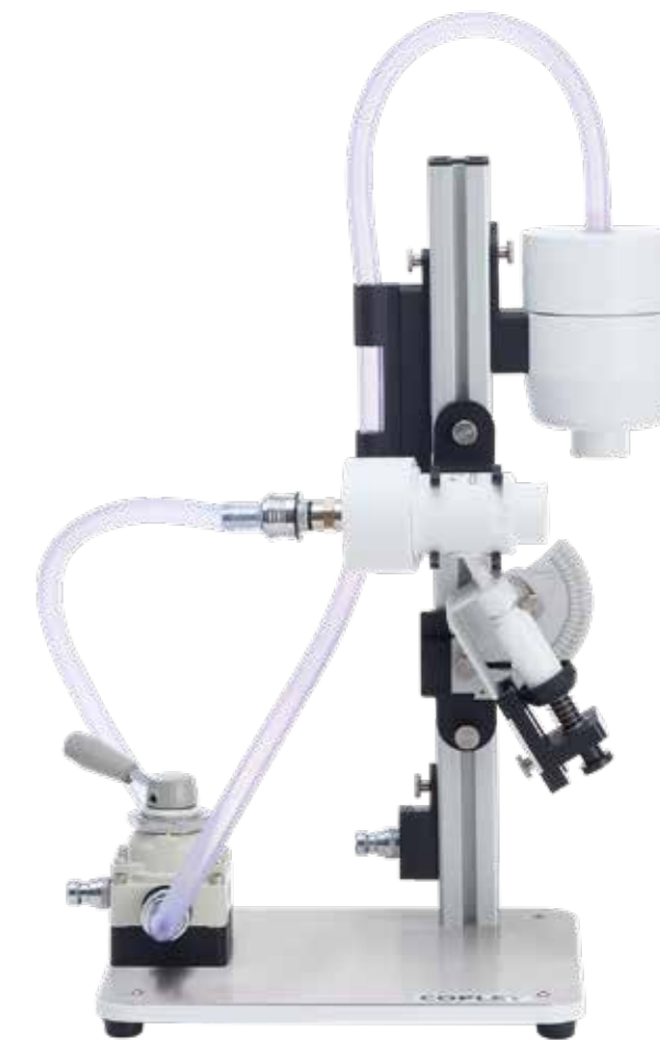
KNI for DDU dose collection with angled nasal device holder
