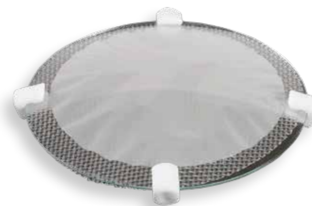
Watchglass/PTFE Assembly for use with ACI
