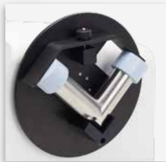
Fixture with ACI/Albuterol Induction Port
