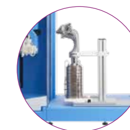
Andersen Cascade Impactor ACI with Alberta Idealised Nasal Inlet AINI
