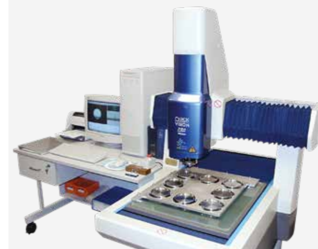
Mensuration of ACI Stages using the Mitutoyo QV404 Vision Inspection System
