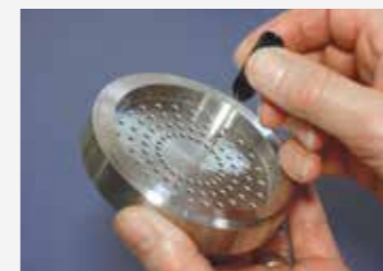
Pinning various stages of the ACI
